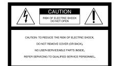
This symbol is intended to alert the user to the presence of uninsulated "dangerous voltage" within the product's enclosure that may be of sufficient magnitude to constitute a risk of electric shock to persons.
